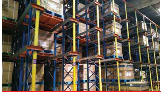
Drive-In Racking System
