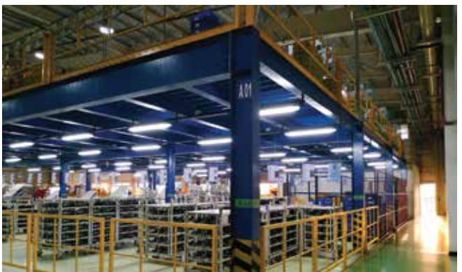
Mezzanine Racking System
