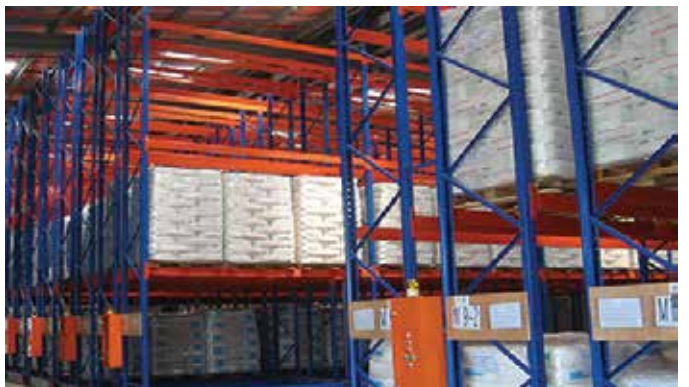
Mobile Racking System
